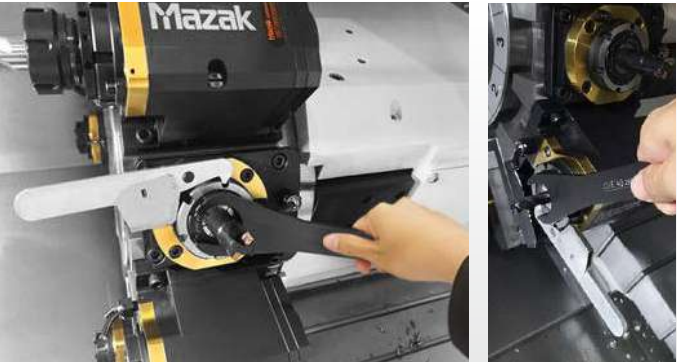
One-hand-wrench can easily tight by spring
