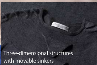
Textured fabric with pin tuck and missed stitches
