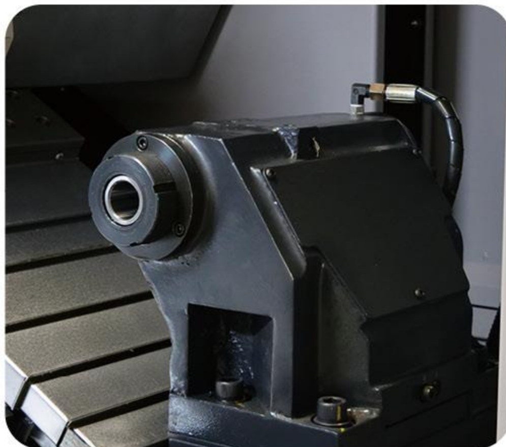
液压尾座 Hydraulic tailstock
